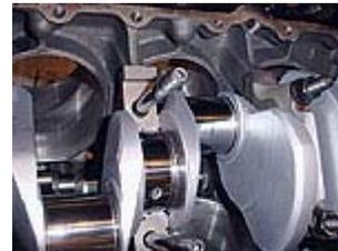
The crankshaft began life in a 330-inch Olds, but went through some changes before ending up at the Jeg's Engine Master Challenge. What a life it's led! The chromed-and-coated piece was machined to a stroke of 3.385-inches. Many feel the 330 steel cranks are too rare, but Dick always seems to have a few on hand. He's also got SFI-certified flywheels drilled in 330 and 425 Olds bolt patterns.
