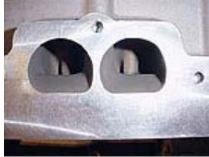
...If the performance of the 403 is any indicator, Olds fans will be happy to see these new heads! We like the line-of-sight intake port design, the efficient D-port exhaust port, and the efficiently-designed combustion chamber...
