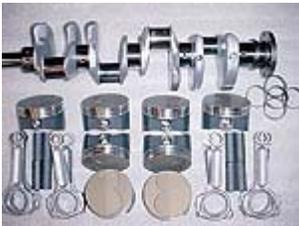
The rotating assembly in this engine looks as good as it works. The pistons, Oliver 6-inch rods, and crank were all coated by Polymer Dynamics (PolyDyn). The crank was treated to lightening, knife edging, and was machined for 2-inch diameter rod bearings. Then, it was chromed (for increased smoothness and less overall drag on the bearings) by Crankshaft Specialist. The crank and rods received PolyDyn's oil shedding coating for less drag and weight while
