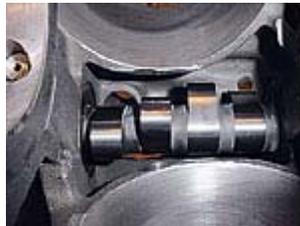
The cam is a custom solid roller ground by Comp Cams (.730/.704-inch lift, 253/256 degrees duration @ .050 on a 107 degree LCA). Dick felt the engine could have used a larger cam. This one ran best with valve lash at .010-inch on the intake side, and .012-inch on the exhaust. With 107-degree lobe separation, the cam was installed with 3 degrees of advance. Dick asked us not to print all the cam specs, since such things are proprietary
