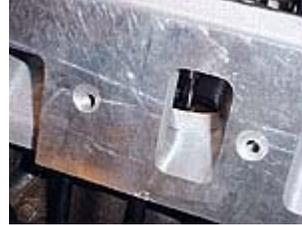
...Again, the coatings are by PolyDyn and these aren't the way the heads ship! This set was worked over by Mike Stark before the chambers and exhaust ports got the thermal barrier treatment.
