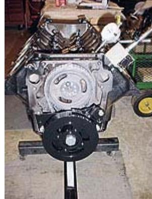
Degreeing in the Comp Cams bumpstick was made easier by using Dick Miller's own DMR-5002 drilled cam degree tool. This is only one of several custom tools Dick has crafted up to make assembling an Olds easier and more effective. We wanted to show you this one in particular, and if you build Olds engines, it oughta be in your toolbox.
