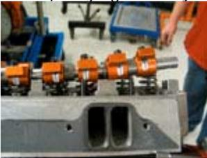
Rocker-arm problems ended Promax's hopes of winning this year's challenge as too short a retaining bolt stripped the threads from the cylinder head allowing the rocker shaft to bend on the first qualifying pull. This was unfortunate for the Promax team because this engine had what could have been a winning combination of power and economy.
