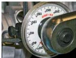
*The 7/16-inch high-tensile ARP 2000 fasteners used in Oliver rods require a special tightening method using a Snap-on torque angle gauge.>*
