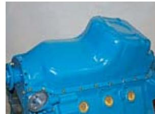
When it comes to Caddy oil pans, there are basically two choices: the rear-sump passenger-car type (shown) or a center-sump pan used on front-wheel-drive Eldorados. The 6-quart (with filter) passenger pan is best for most custom applications. For initial break-in and dyno runs, Miller used Lucas 20W-50 conventional oil. Eventually he'll switch to synthetic.
