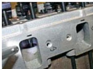
On original Bulldog heads the intake port roof was raised slightly over stock. Stock and Edelbrock intakes still bolt up, but if port-matched, the intake flange thickness is left really
