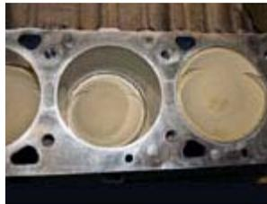
Diamond forged pistons and pins were treated to PolyDyn high-tech coatings: a heat-reflective thermal barrier on the piston deck and antisuff dry-film lubricants on the piston skirt and piston pins.
