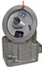
To ensure all oil passes through his K&N filter, Miller removed the stock oil-pump plastic bypass valve, drilling and tapping its orifice for a socket-head pipe plug (arrow). JB Weld provides added insurance.
