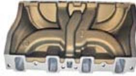
Creative Flow Management port-matched Edelbrock's Performer Cadillac dual-plane (PN 2115). The spread-bore intake is designed to make low- and midrange torque through 5,500 rpm. PolyDyn thermal-barrier piston stroke. Holley's PN 12-150 coatings were applied to the valley side to prevent hot oil from heating the air/fuel charge.
