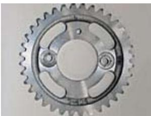
With no separate dowel pin like in a Chevy, to advance or retard a Caddy cam you must drill both sprocket mounting-bolt holes oversize and install bushings in each hole. Miller's bushing kit (PN DMR-5155-C) was installed with red thread-locking compound, then staked in place.
