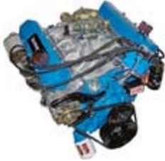
*It's not your grandpa's Cadillac engine. Dick Miller's 541ci Caddy stroker uses newly developed heads plus a custom Comp Cams bumpstick and valvetrain to produce tons of tire-twisting torque at a realistic engine speed.>*
