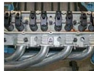
MTS Bulldog heads accept the stock Caddy valvetrain, aftermarket shaft-mount systems, or stud-mounted rockers. Miller used adjustable Comp Cams 1.7:1 aluminum full-roller stud-mount rockers listed for a [Ford 289/302/351W](#) (PN 1049-16).
