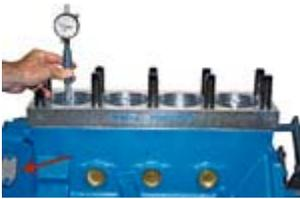
Up to 0.120-inch overbores are usually OK on a Caddy without block filler, although a copper gasket is needed over 0.080. This engine is 0.075-over. Yes, BHJ makes a Caddy torque plate (PN 472/500-R-S-AL-T). Miller offers the stainless fuel-pump block-off (PN DMR-5950-C, arrow).
