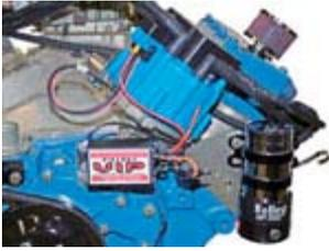
Performance Distributors' DUI distributor (PN 817211) and Live Wires (PN C9075) receive 18 volts from a VIP step-up box (PN 5577). The extra juice allows wide-gapping of the spark plugs for a more powerful burn on each rpm. PolyDyn thermal-barrier piston stroke. Holley's PN 12-150 coatings were applied to the 150-gph electric fuel pump is used in place of the inadequate Caddy mechanical fuel pump.
