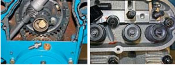
An antiwalk button is used to fight the cam's tendency to push forward under load. To set the clearance, file the bolt (not the bronze bushing) in Miller's kit (PN DMR-5740-C). Check by laying a straightedge across the front cover gasket, wedging the cam rearward, and inserting a feeler gauge. Miller's two-piece front cover (PN DMR-2582-C) allows cam changes without damper removal or disturbing the pan gasket.
