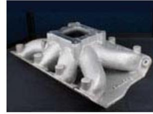
For higher-rpm applications, check out MTS' single-plane intake. Recent versions have a smaller plenum to optimize 2,500- to 6,500-rpm performance. Larger variants are available with standard Holley, 4500 Dominator, or Q-Jet mounting flanges. You can drill the blank cast-in bosses for EFI or nitrous nozzles.
