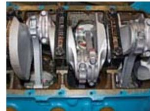
The piston pins hang on the rods using floating pins retained by double 0.042-inch Spirollocks. The stroker parts drop right into the Caddy block-no need for clearance grinding. At this power level, the two-bolt bottom end needs help from Miller's new billet main caps retained by ARP studs (complete Miller stud-and-cap kit, PN DMR-5943-C-S).
